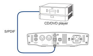
Connect your digital source (ex. CD/DVD players or some PC/NB with SPDIF output) to Digital Input. Either S/P DIF Coaxial or Toslink optical types can be used, each being of equal quality.
