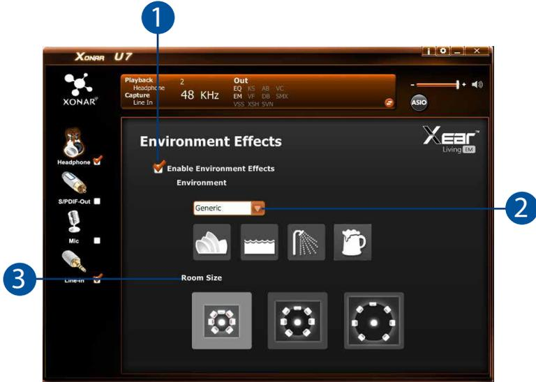
This function provides 28 special environment emulations for different sound reflections and reverberation.
