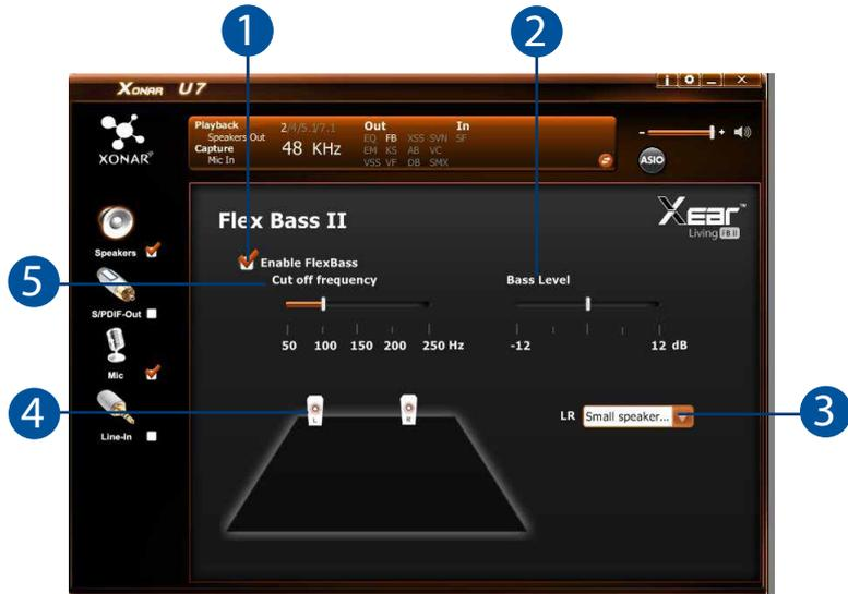
This function allows you to increase / decrease the LFE strength. This function would cut the low frequency band (50~250Hz) of stereo music content (eg. Mp3,WMA, CD Audio) and transfer to subwoofer or each speaker.
