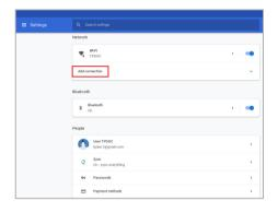
Choose Add Wi-Fi... then input the necessary details to setup your new network connection.
