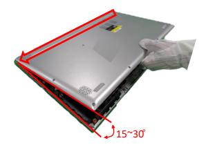
H. Put the base cover down slowly, and then press left and right side of base cover to fix, and press lower side of base cover to fix.
