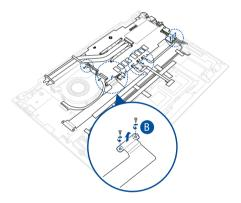
D. Remove the screw(s) from the motherboard and then remove the motherboard from the chassis.
