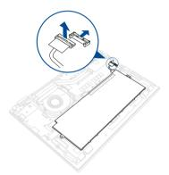
To connect the battery, align and connect the cable to the battery connector before you reattach the compartment cover.
