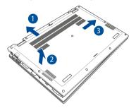
**IMPORTANT!** Cables are connected. Avoid damaging the cable connectors when removing the compartment cover.
