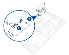
D. Remove the M.2 SSD module from the motherboard.
