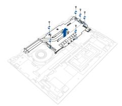
E. Remove the screw(s) from the cooling radiator.
