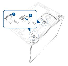
E. Remove the screw(s) from the hinges, and then remove the LCD panel module.
