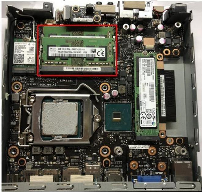
2. Push the slot latch on both sides.
