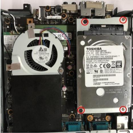
2: Disconnect the HDD connect cable.
