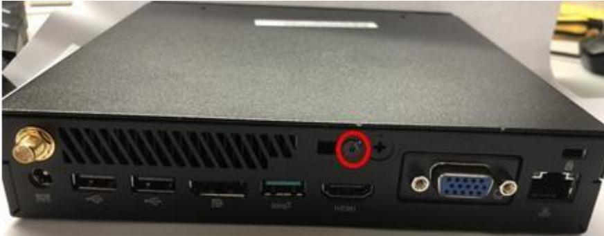
2: Push the Bottom Cover by following the red direction, and make it to be not locked.
