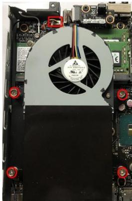
3: Remove the Thermal Module.
