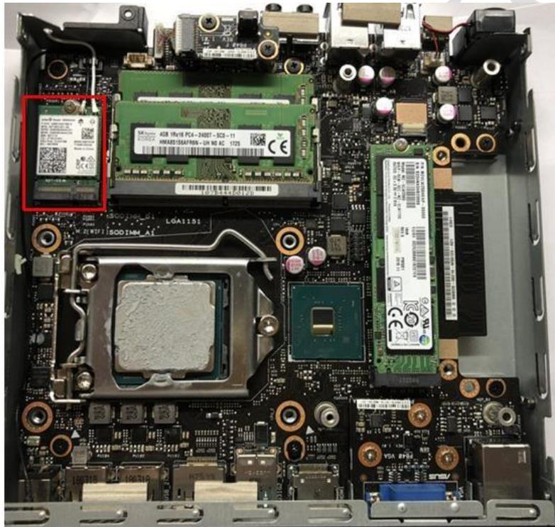
3: Disconnect the RF Cable and remove the screw (M2\*3L).
