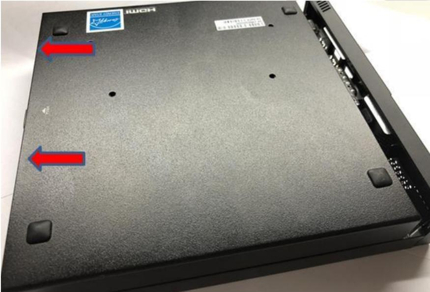
3: Lift the Bottom Cover from the no-locked side.
