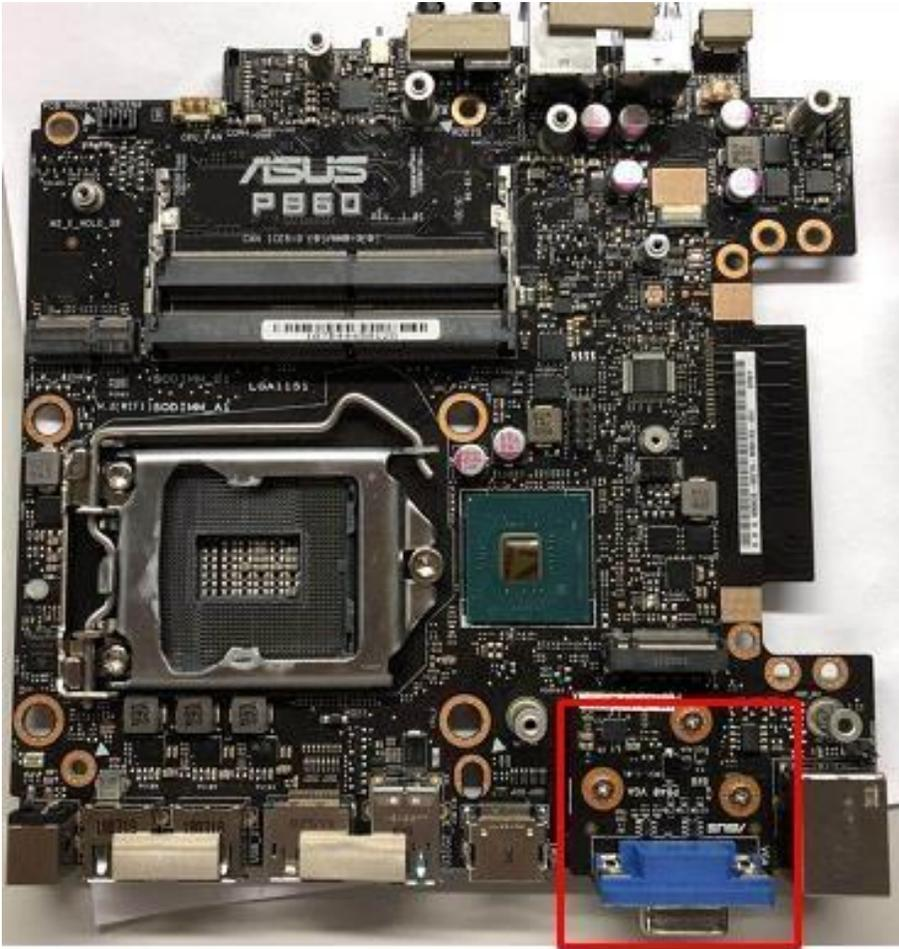
2: Remove 3 screws (M2\*3L), and remove the VGA Board.
