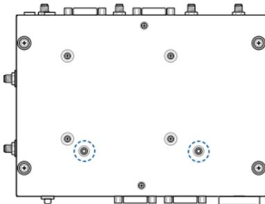
3. Remove the screw hole covers at the back of your VESA mount-compatible device, if they exist.
