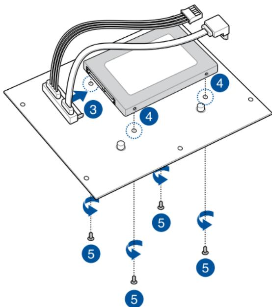
6. Connect the storage device cable to the **SATA6G** and **SATA\_PWR** connectors on the motherboard.
