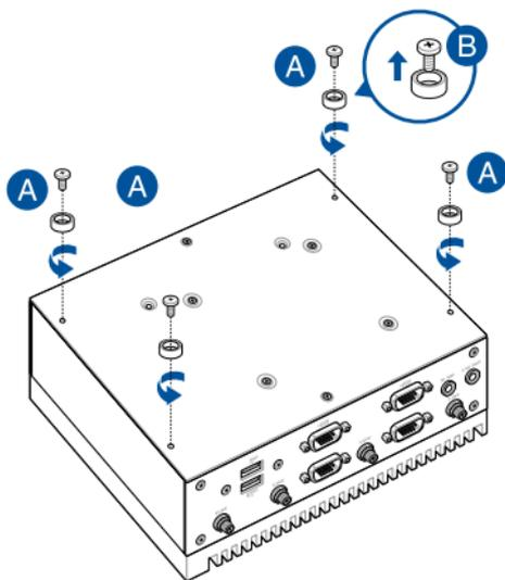
2. Align the wall mount with the rubber feet screw holes (A), and then secure the wall mount brackets to your Embedded Computer using the rubber feet screws (B).
