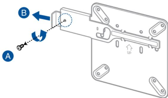
7. Position the Embedded Computer and insert the screws attached on the Embedded Computer to the mounting holes of the VESA mounting plate (A), then gently push the Embedded Computer down in the angle shown in the illustration to secure it in place (B).
