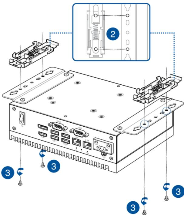
4. Clip the final assembly to a DIN rail by hooking the DIN rail clips to the top of the DIN rail and then pressing down until you hear the clips snap into place.
