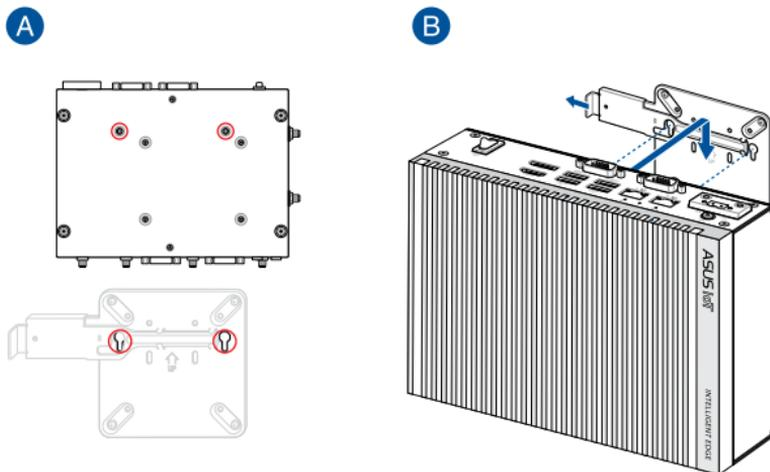
8. Push the metal lock back towards the Embedded Computer (A), and then secure it using the screw previously removed (B).
