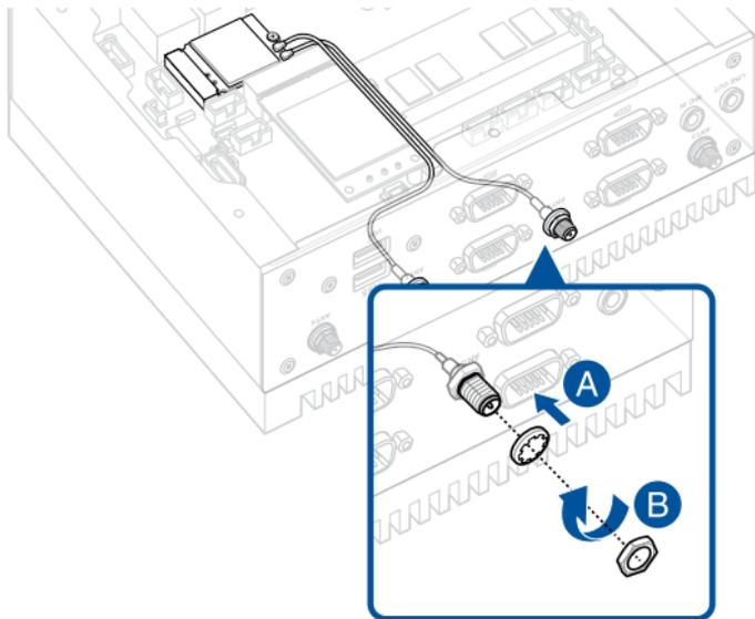
6. Connect the other end of the RF connector and cable to your wireless card (refer to **Installing a wireless card to the M.2 (E-key) slot** for details) or to your WWAN card (refer to **Installing an mPCIe / mSATA module** for details).
