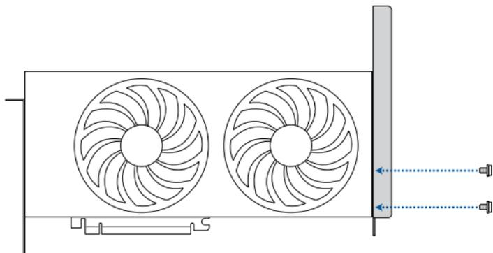
2. Insert your GPU card to the empty PCIe slot corresponding to the punch-out port(s) with the metal cover(s) you removed earlier, and ensure that it is securely seated in the slot.
