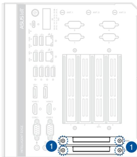
3. Install your storage device to the storage device tray, then secure it with four (4) screws.
