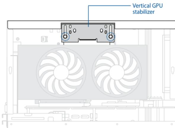
5. Move the vertical GPU stabilizer down until it rests securely on top of the GPU card (A), and secure it to the GPU support plate with two (2) screws.
