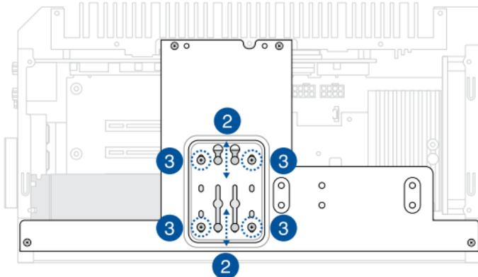
4. Fit the bottom rounded end of the slotted holes on the vertical GPU stabilizer over the two retaining pins on the side of the GPU support plate as shown.
