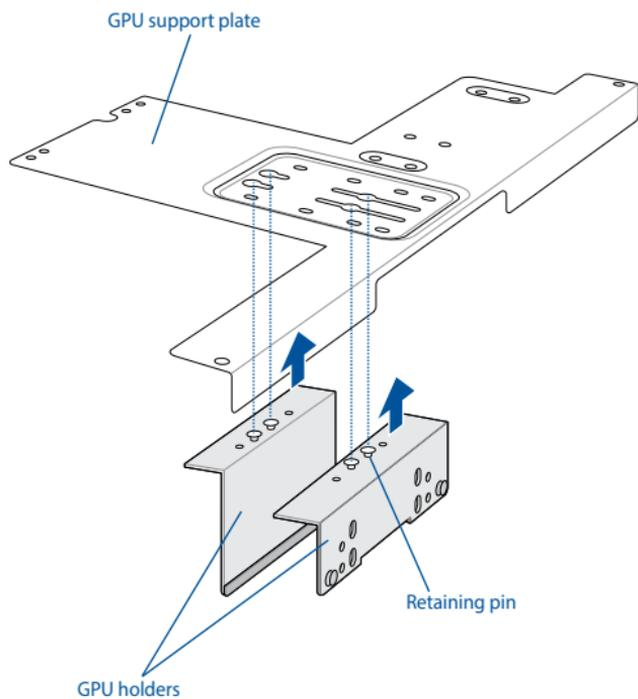
2. Slide the two GPU holders so that they are positioned as closely as possible to both sides of the GPU card to provide support.
