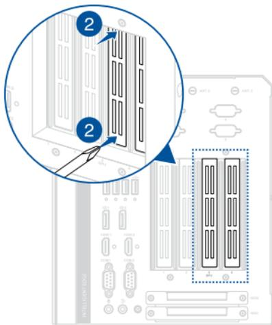
3. Carefully remove the detached metal cover from the chassis.
