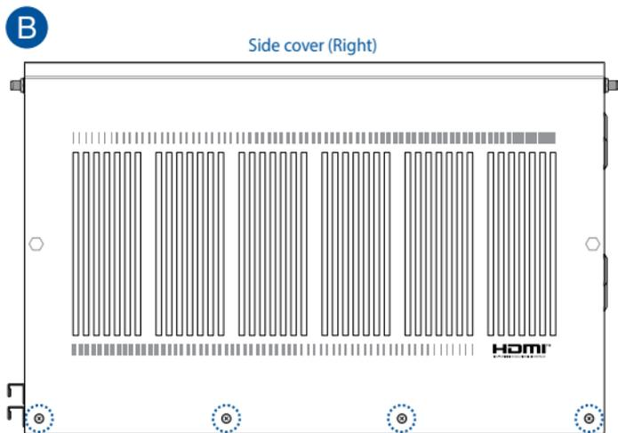
4. Lift the side cover to clear the two (2) knobs from the slotted holes on the chassis, then move it away from the chassis to remove it.
