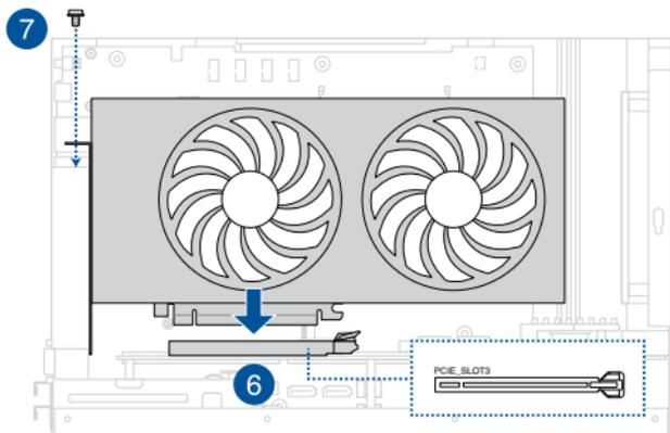
8. Depending on your GPU card's power requirements, you may need to connect one or two power cables from the riser board to your GPU card. Connect one end of the power cable(s) that came with your GPU card to the expansion card (A) and the other end to the PCIe riser board (B).
