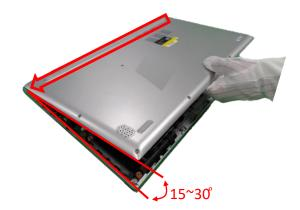
J. Put the base cover down slowly, and then press left and right side of base cover to fix, and press lower side of base cover to fix.
