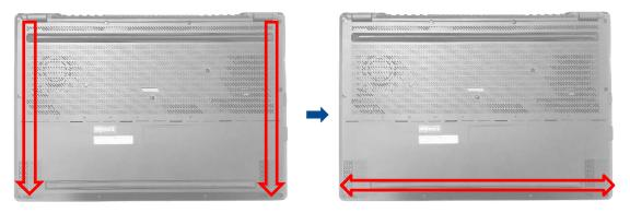
K. Secure the base cover in place using the screws.
