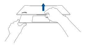
**NOTE:** For better heat dissipation, we recommend that you open the display panel to at least 60 degrees while in use.
