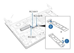
**NOTE:** The M.2 2280 slot II supports PCIe (NVMe) SSD while slot I and slot III support both PCIe (NVMe) SSD and SATA SSD.
