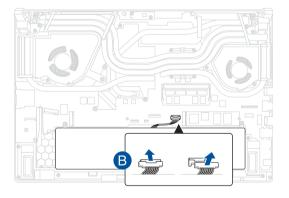
To connect the battery, align and connect the cable to the battery connector before you reattach the compartment cover.
