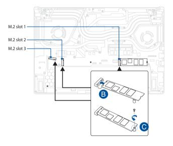
${\bf NOTE:}$  The M.2 2280 slot 1 and slot 3 support PCle (NVMe) SSD while slot 2 supports both PCle (NVMe) SSD and SATA SSD.
