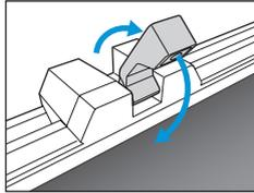
2. When the color sensor reaches the edge of the screen, it will stop and start the calibration process. The calibration time depends on the amount of preset modes you select, the longest time might be 30 minutes.
