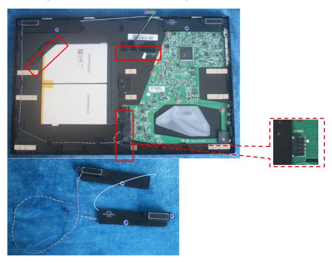
2. Remove the Battery: Pull the black Mylar handle directly, then pull it out evenly to separate the battery, and disconnect the Battery connector
