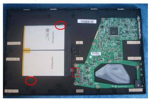
3. Unscrew the screws to remove the Main Board
