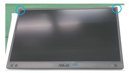
3. Press four sides follow the sequence (1-2-3) as below. Take care to protect the BEZEL. Please check whether the bezel is assembled properly after assembling and make sure the BEZEL is not damaged.
