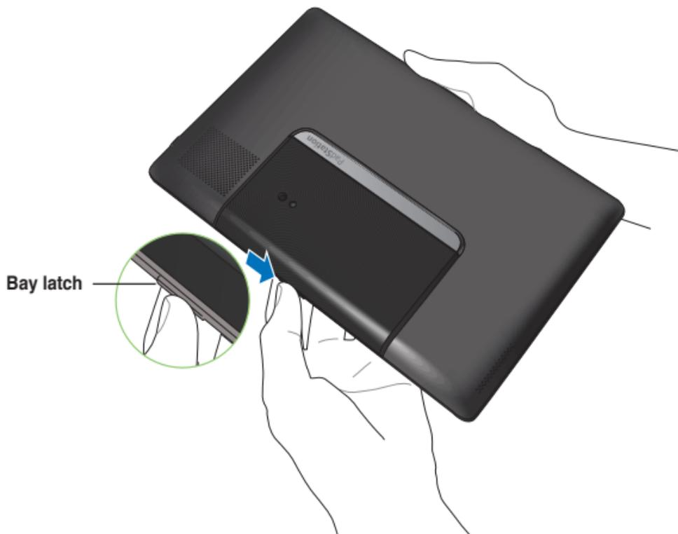
2. Push the PadFone bay door up to a ninety-degree (90°) angle until the PadFone detaches completely from the connectors.
