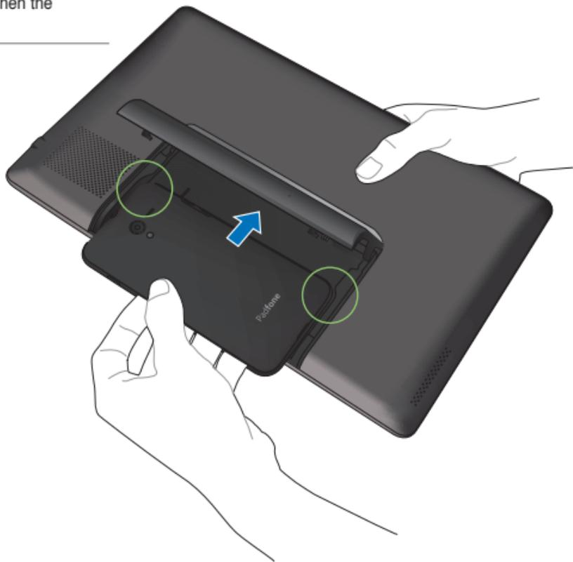
4. Close the PadFone bay door and ensure that the latch firmly locks in place.
