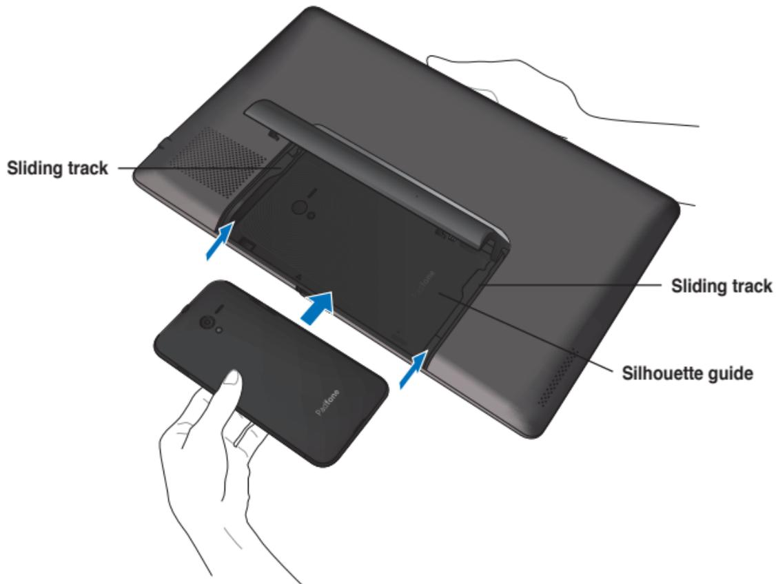
3. Firmly insert your PadFone into the PadFone Station until the PadFone is secured in place.
