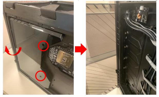
3. Lift the cable cover panel upwards to remove.
