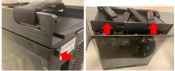
2. Remove the two screws on the cable cover panel, open it up to a 90-degree angle, and then lift it upwards to remove.
