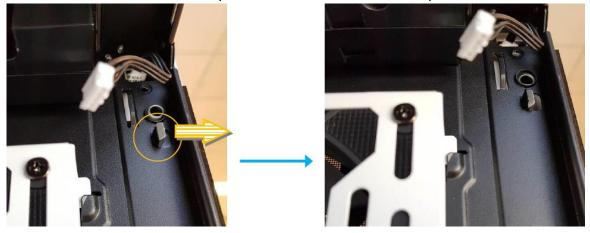
5. Remove the left side panel from the chassis and pull out the left LED cable through the hole on the top of the chassis.
