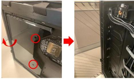
3. Disconnect the cables connected to the motherboard.
