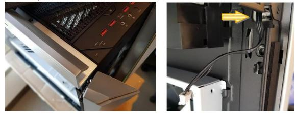
6. Pull the left side panel outward from top to bottom until it completely detaches from the front glass.
