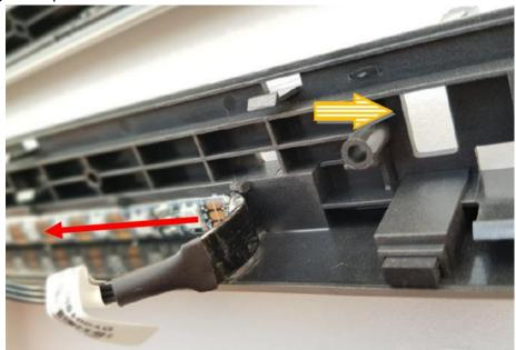
10. Install the new LED strip by aligning the end of the strip with the side wall and gradually sticking it upwards after removing the backing paper.
