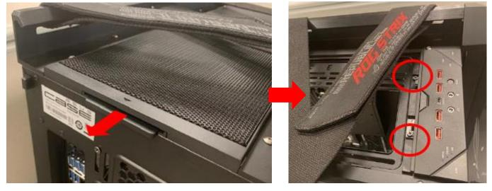
8. Press the front latch to remove and replace the FIO module.
