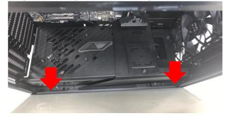
3. After closing the glass panel, it will be locked automatically.
