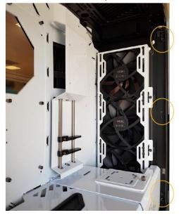
4. Gently push the hook on the upper side of the left side panel towards the outside of the chassis to loosen and detach the plastic hook from the metal piece.
