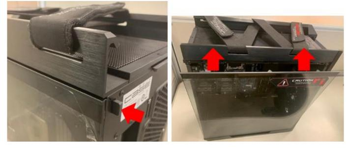
2. Remove the two screws on the cable cover panel, then open it up to a 90-degree angle.
