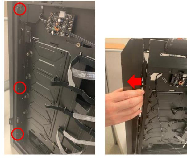
5. Separate the panel from the front glass (be careful to hold the front glass to prevent it from falling).
