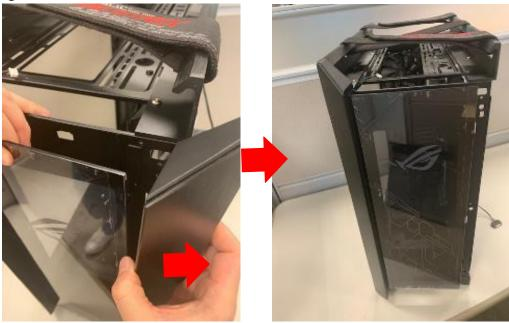
6. Remove the other two screws on the opposite side while holding the front glass to prevent it from falling, then take out the front glass for replacement.
