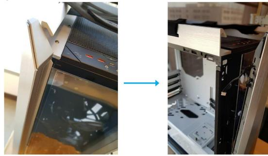
7. Place the ASUS accessory box under the glass to prevent the glass from suddenly detaching or getting damaged.
