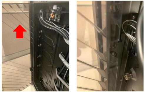
4. Remove three screws to pull out the front panel.
