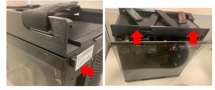
1. Press the rear switch and lift the damaged glass panel.
