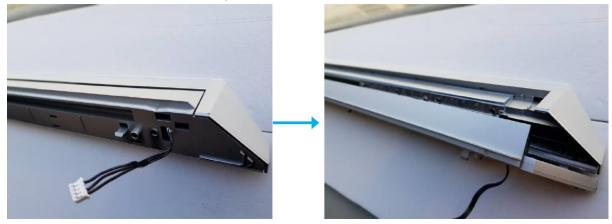
9. Tear off the LED light strip, after the wire head pass through the square hole in the plastic piece, the light strip can be torn to the end.
