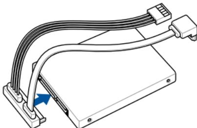
2. Connect the storage device cable to the **SATA6G** and **SATA\_PWR** connectors on the motherboard.
