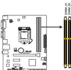
B85M-F 240-pin DDR3 DIMM sockets
