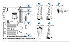
Do not forget to connect the fan cables to the fan connectors. Insufficient air flow inside the system may damage the motherboard components. These are not jumpers! Do not place jumper caps on the fan connectors! The CPU\_FAN connector supports a CPU fan of maximum 1 A (12 W) fan power.
