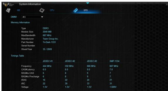
The screenshot shows the 'System Information' window with the 'SPD' tab selected. It displays memory details for DIMM #1, including type, size, bandwidth, manufacturer, and a timing table.
