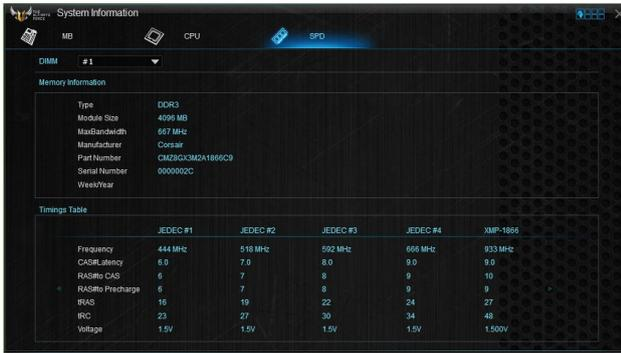
The screenshot shows the 'System Information' window with the 'SPD' tab selected. It displays memory details for DIMM #1, including type (DDR3), capacity (4096 MB), and manufacturer (Corsair). Below this is a 'Timings Table' with columns for JEDEC #1, JEDEC #2, JEDEC #3, JEDEC #4, and XMP-1866, and rows for Frequency, CAS# Latency, RAS#to CAS#, RAS#to Precharge, tRAS, tRC, and Voltage.
