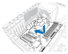
Place six screws into the holes indicated by circles to secure the motherboard to the chassis.
