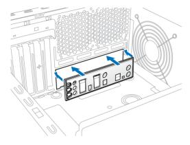
2. Place the motherboard into the chassis, ensuring that its rear I/O ports are aligned to the chassis' rear I/O panel.
