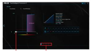
Click and drag to adjust the fan's speed CPU and chassis fan screens
