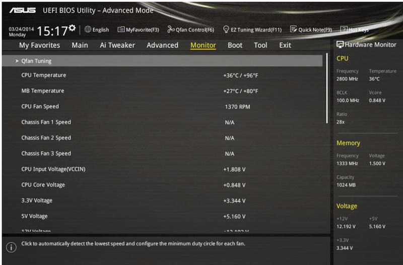
Click to automatically detect the lowest speed and configure the minimum duty circle for each fan.
