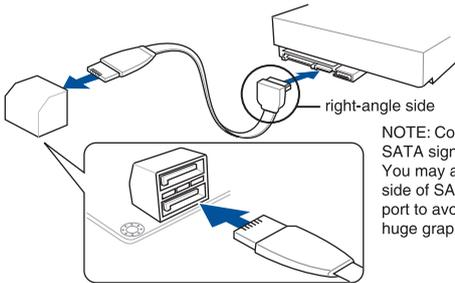
NOTE: Connect the right-angle side of SATA signal cable to SATA device. You may also connect the right-angle side of SATA cable to the onboard SATA port to avoid mechanical conflict with huge graphics cards.
