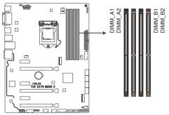
TUF Z270 MARK 2 288-pin DDR4 DIMM socket
