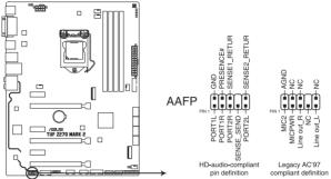
TUF Z270 MARK 2 Analog front panel connector
