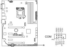
TUF Z270 MARK 2 Serial port connector
