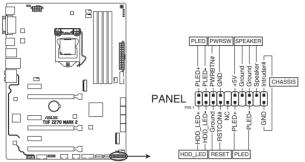
TUF Z270 MARK 2 System panel connector
