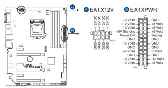
**TUF Z270 MARK 2 ATX power connectors**
