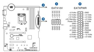
**TUF Z370-PLUS GAMING II ATX power connectors**
