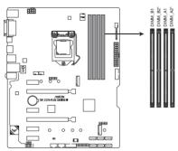
TUF Z370-PLUS GAMING II 288-pin DDR4 DIMM sockets
