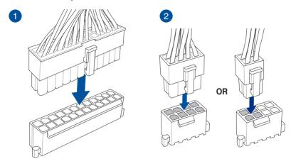
Ensure to connect the 8-pin power plug.
