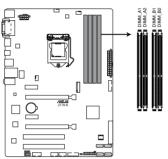
Z170-K 288-pin DDR4 DIMM sockets
