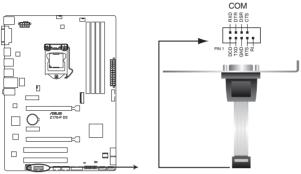
Z170-P D3 Serial port (COM) connector
