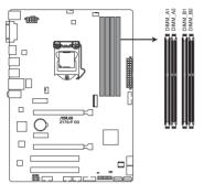
Z170-P D3 240-pin DDR3 DIMM sockets
