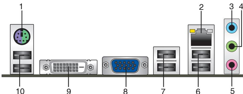
1. **PS/2 Keyboard / Mouse Combo port.** This port is for a PS/2 keyboard or PS/2 mouse.
