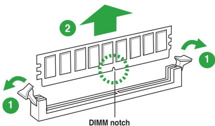
2. Remove the DIMM from the socket.
