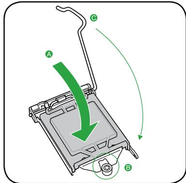
6. Insert the load lever under the retention tab.
