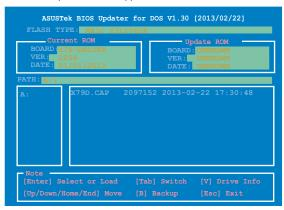
Press <Tab> to switch between screen fields and use the <Up/Down/Home/End> keys
