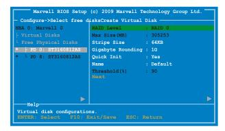
Use the up or down arrow key to move the selection bar and press <Enter> to configure further RAID settings.
