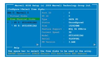
Press <Space> to select the hard drives to be included in the RAID array. An asterisk
