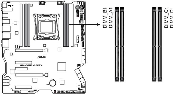
RAMPAGE VI APEX 288-pin DDR4 DIMM socket
