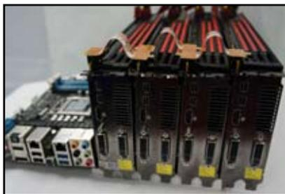
5. Connect four independent auxiliary power sources from the power supply to the four graphics cards separately.
