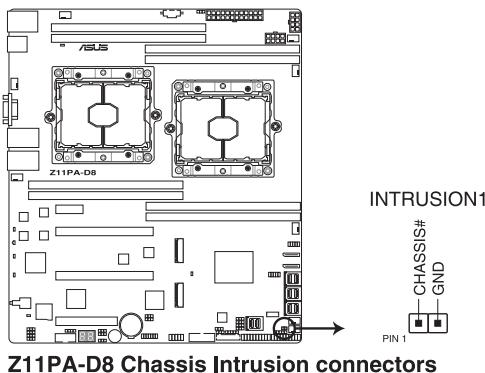
Z11PA-D8 Chassis Intrusion connectors
