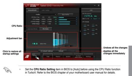
The CPU Ratio bars show the status of the CPU cores, which vary with your CPU model.
