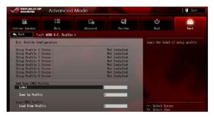
The O.C. Profile Configuration items show Not Installed if no profile is created.
