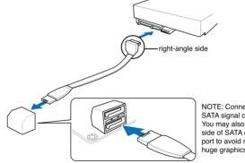
NOTE: Connect the right-angle side of SATA signal cable to SATA device. You may also connect the right-angle side of SATA cable to the onboard SATA port to avoid mechanical conflict with huge graphics cards.
