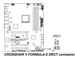
Ensure that your chassis comes with the button cable that supports the DirectKey feature. Refer to the technical documentation that came with the chassis for details.
