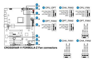
DO NOT forget to connect the fan cables to the fan connectors. Insufficient air flow inside the system may damage the motherboard components. These are not jumpers! Do not place jumper caps on the fan connectors!
