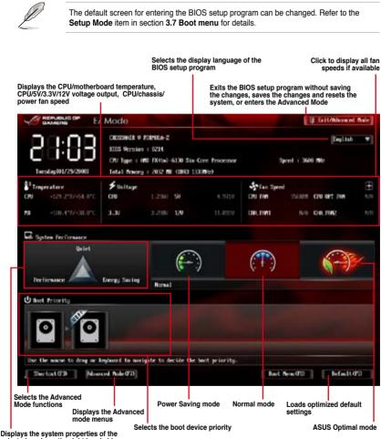
Displays the system properties of the selected mode on the right hand side
