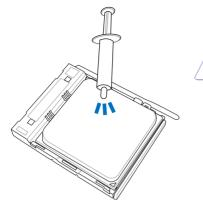
Apply the Thermal Interface Material to the CPU heatsink and CPU before you install the heatsink and fan if necessary.
