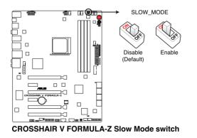
Ensure to set the LN2 Mode jumper to [Enable] before using the Slow Mode Switch.
