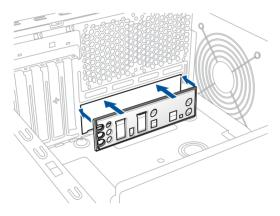
Place the motherboard into the chassis, ensuring that its rear I/O ports are aligned to the chassis' rear I/O panel.
