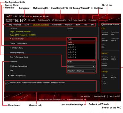
Displays the CPU temperature, CPU, and memory voltage output
