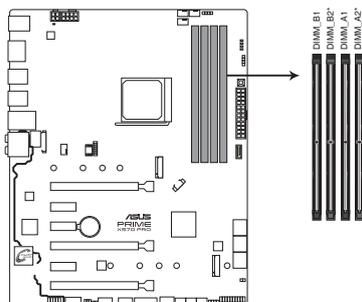
**PRIME X570-PRO 288-pin DDR4 DIMM sockets**
