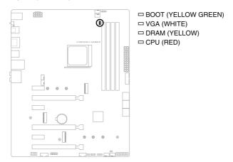
The Q-LEDs provide the most probable cause of an error code as a starting point for troubleshooting. The actual cause may vary from case to case.
