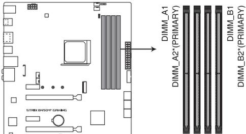
**ROG STRIX B450-F GAMING 288-pin DDR4 DIMM socket**
