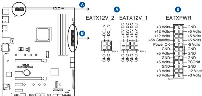
TUF GAMING X570-PLUS ATX power connectors
