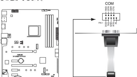
TUF GAMING X570-PLUS Serial port (COM) connector
