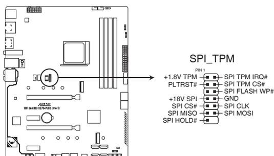
**TUF GAMING X570-PLUS (WI-FI) SPI\_TPM connector**
