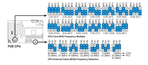
**WARNING!** Frequencies above 100MHz exceed the specifications for the onboard Intel Chipset and are not guaranteed to be stable.
