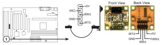
**P2B Infrared Module Connector**
