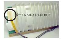
**WARNING!** Do not insert the sensor between the processor and heatsink, otherwise, it will cause damage to the P2T-Cable.
