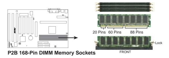
The DIMMs must be 3.3Volt unbuffered SDRAMs. To determine the DIMM type, check the notches on the DIMMs (see figure below).
