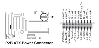
**IMPORTANT:** Make sure that your ATX power supply can supply at least 10mAmp on the 5-volt standby lead (5VSB). You may experience difficulty in powering on your system if your power supply cannot support the load. For Wake on LAN support, your ATX power supply must supply at least 720mA.
