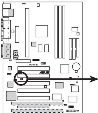
**IMPORTANT:** Requires an ATX power supply with at least 720mA +5 volt standby power
