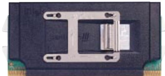
Example of an incorrectly installed retention clip
