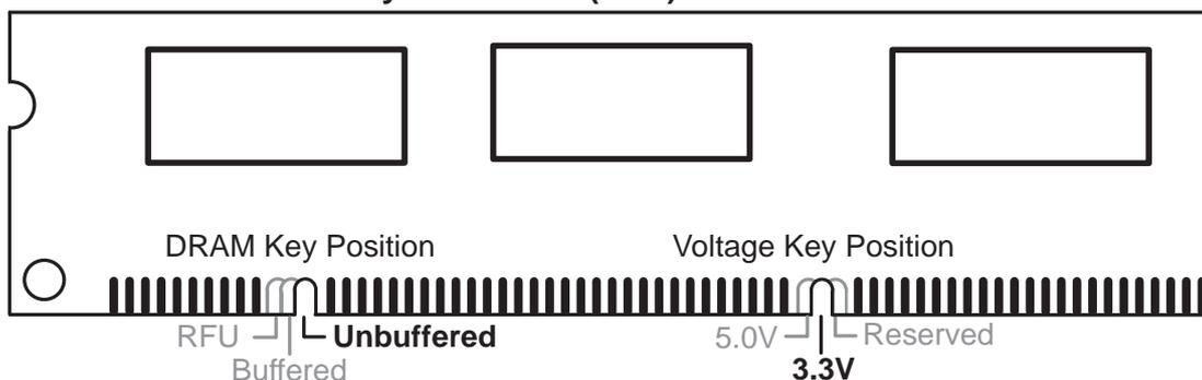
The notches on the DIMM module will shift between left, center, or right to identify the type and also to prevent the wrong type from being inserted into the DIMM slot on the motherboard. You must ask your retailer the correct DIMM type before purchasing. This motherboard supports four clock signals per DIMM slot.
