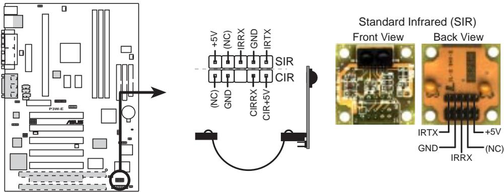
**P3W-E Infrared Module Connector**
