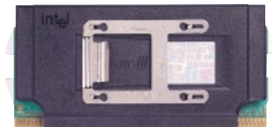
Example of an incorrectly installed retention clip
