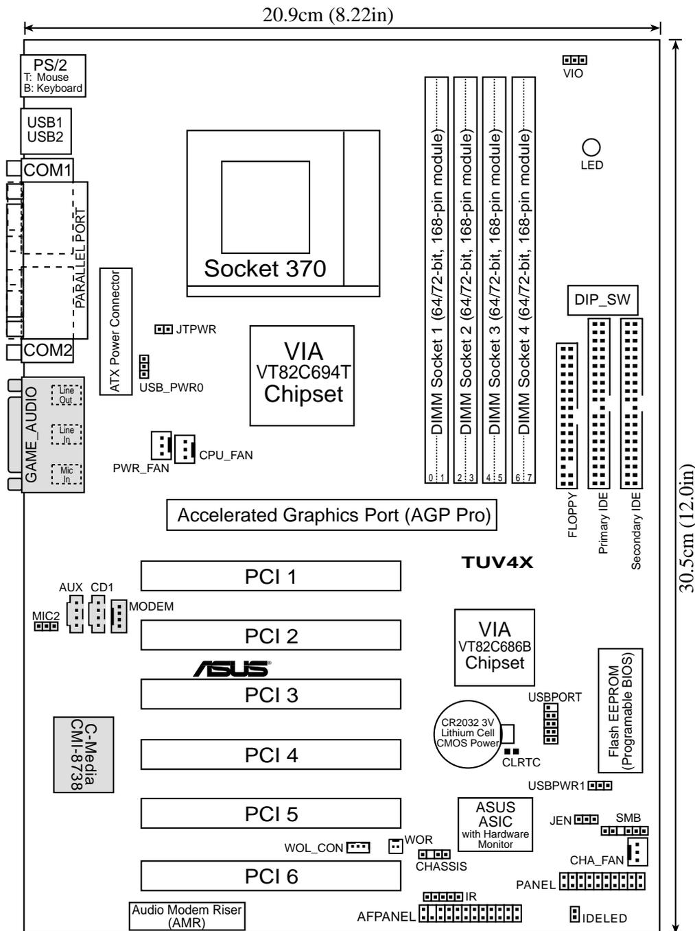
**NOTE:** The audio chipset, external GAME/AUDIO connectors, and internal audio connectors are optional components, and present in audio models only. The components are grayed in the above motherboard layout.
