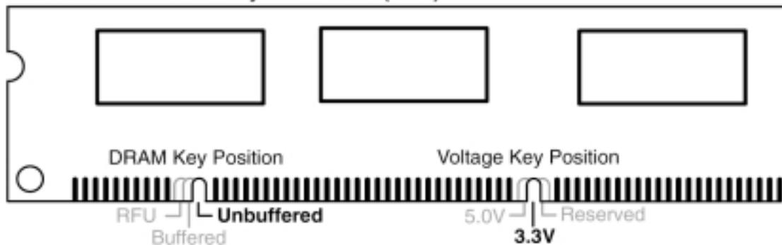
The notches on the DIMM shifts between left, center, or right to identify the type and also to prevent the wrong type from being inserted into the DIMM slot on the motherboard. You must tell your retailer the correct DIMM type before purchasing. This motherboard supports four clock signals per DIMM.
