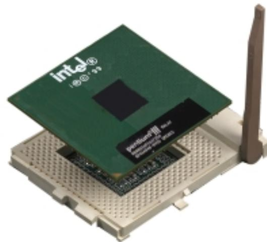
**CAUTION!** The CPU fits only in one orientation. Do not force the CPU into the socket to prevent bending the pins and damaging the CPU. If the CPU does not fit completely, check its orientation or check for bent pins.
