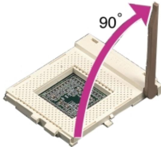
3. Position the CPU above the socket such that its notched or marked corner matches the socket corner near the end of the lever, while making sure that the CPU is parallel to the socket.
