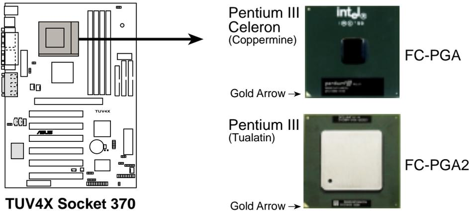
Note in the illustration that CPUs have marks (usually a notch or a gold mark on one corner) to help you identify the proper orientation and enable you to correctly install a CPU. It is important that you match the marked corner of the CPU with the corresponding corner on the socket so as not to damage the CPU pins.
