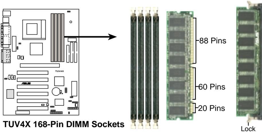
The DIMMs must be 3.3Volt unbuffered SDRAMs. To determine the DIMM type, check the notches on the DIMMs (see the figure below).
