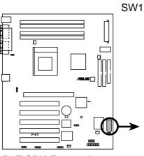
P4T CPU External Clock (BUS) Frequency Selection
