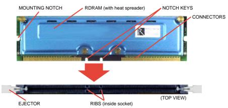
2. With the ejectors in the open position (as shown), push down gently but firmly on the memory module until it snaps into place. The guides on the socket's ejectors should go through the two mounting notches on the module and the ejectors should close. If necessary, push the ejectors inward to secure the module in place.
