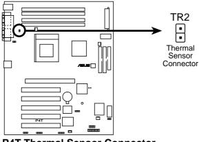
P4T Thermal Sensor Connector
