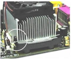
2. Connect the *CPU fan cable* to the *fan connector*. (*See 3.1 Motherboard Layout / 3.8 Connectors*).
