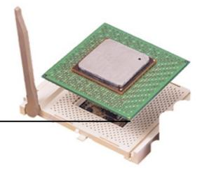
3. Once completely inserted, press the CPU firmly and close the socket lever until it snaps into its locked position.
