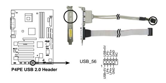
NEVER connect a **1394 cable** to the USB\_56 connector. Doing so will damage the motherboard!
