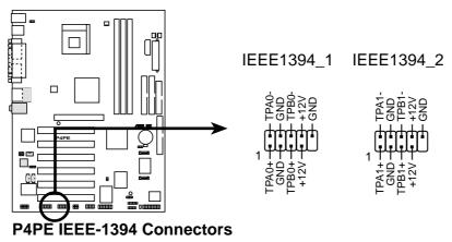
NEVER connect a **USB cable** to any of the IEEE 1394 connectors. Doing so will damage the motherboard!
