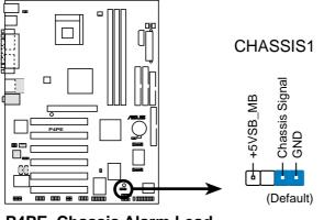
P4PE Chassis Alarm Lead
