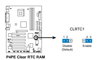
You do not need to clear the RTC when the system hangs due to overclocking. For system failure due to overclocking, use the C.P.R. (CPU Parameter Recall) feature. Shut down and reboot the system so BIOS can automatically reset parameter settings to default values.
