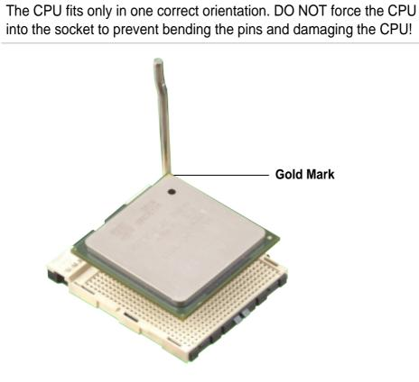
5. When the CPU is in place, push down the socket lever to secure the CPU. The lever clicks on the side tab to indicate that it is locked.
