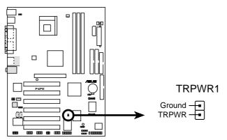
P4PE Power Supply Thermal Connector
