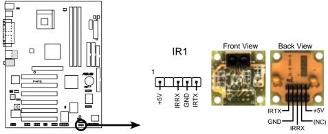
P4PE Infrared Module Connector
