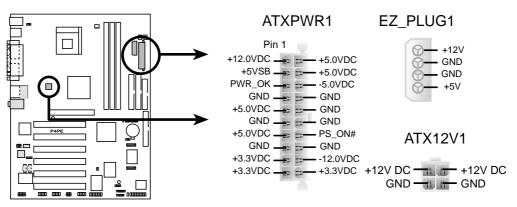
P4PE ATX & Auxiliary Power Connectors
