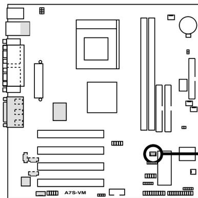
**IMPORTANT:** Requires an ATX power supply with at least 720mA +5 volt standby power
