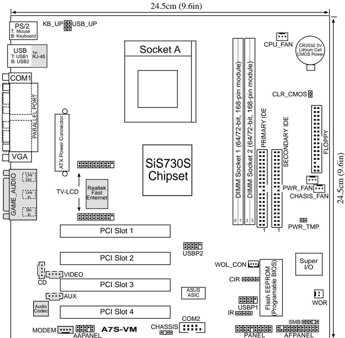
**NOTE:** The Audio Codec, external and internal audio connectors, RealTek RTL8100 chipset, and RJ-45 LAN connector are optional components. These items are grayed out in the above motherboard layout.
