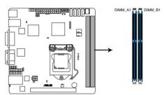
P9D-I 240-pin DDR3 DIMM sockets
